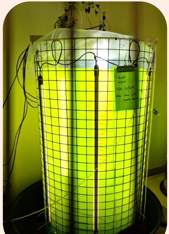
Prototype algal bioreactor with light and internal sensors. The light distribution, gas transfer and fluid dynamics are being modelled to improve production.
